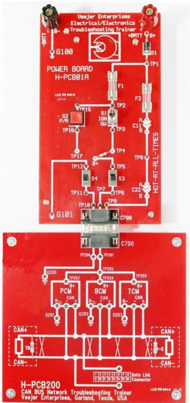
To learn to repair CAN Bus problems you must have specific electrical troubleshooting skills of CAN Bus wiring network problems as well as the best procedure to troubleshoot the voltage circuits (B+) and ground circuits (B-) supplying the Nodes. This training program provides specific CAN Bus system troubleshooting scenarios. The CAN Bus Trainer, **H-PCB200**, is shown below connected to the Power Board from the Starter Kit, H-111A.
