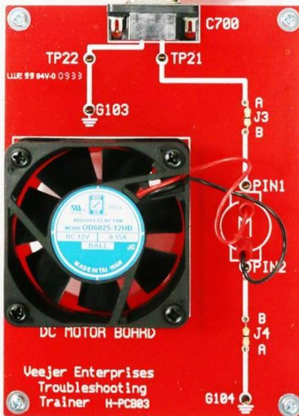
The DC Motor circuit is described as an **engine cooling fan** circuit to add realism to the troubleshooting problems. Circuit electrical problems inserted are open circuits, voltage drops on the voltage-side or the ground-side of the circuit, short-to-ground and short-to-voltage problems. Several problems deal with advanced ground-side failures. Follow these troubleshooting procedures and breeze through ground-side problems in any vehicle circuit.
